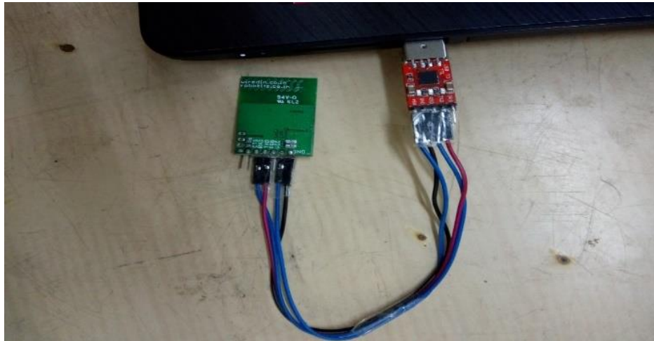
Fig 11: Arduino interfacing with hexapod
